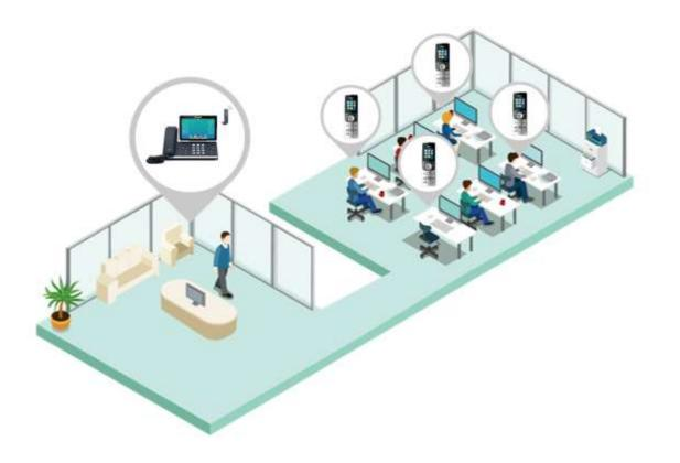
Clone Mode (T5W is Master and the handset is Slave): Support seamless call switchover between the desktop phone and the DECT handset (only when one DECT handset is registered)
